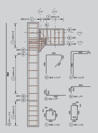
SOFiSTiK Reinforcement significantly accelerates the creation of 2D reinforcement sheets out of 3D- Rebar models in Autodesk<sup>®</sup> Revit<sup>®</sup>.
